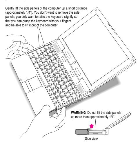
8 Carefully pull the keyboard forward to loosen the four tabs at the top. Be very careful to avoid pulling the keyboard out too far. The cable attaching the keyboard to the computer is very short.
